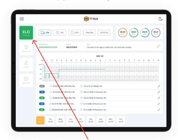
If the ELD is connected to vehicle driver can see green icon on top right side of dashboard.
